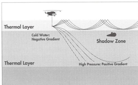
**Figure 6.1: Thermal Layers**
