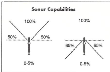
**Figure 5.6: Increased Sonar Capabilities With Towed Array**
